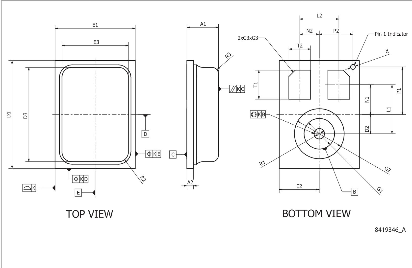
Table 6. RHLGA metal cap 3-lead (3.35 x 2.5 x 0.98 mm) package dimensions
