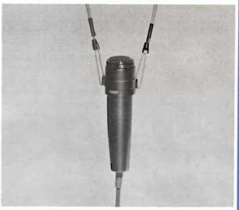
A low-impedance balanced-output unit, the D-109 is supplied complete with a 9 m ( $\approx$ 29-1/2 ft) flexible, 2-conductor shielded cable having stripped and tinned leads at its free end. (The cable is an integral part of the microphone, but can be easily replaced in the field.) Also included are the lavalier clip (with adjustable tie clasp and adjustable/removable nylon neck cord) and a foam-lined vinyl protective case.
