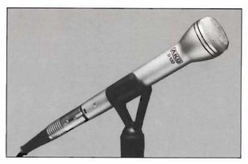
further precaution, the transducer incorporates a hum-bucking winding to cancel the effects of stray magnetic fields. The microphone's sintered-bronze windscreen (an AKG exclusive) and impact-resistant zinc-alloy case encapsulate all internal parts against metal particles, dust and moisture spray. Should field service ever become necessary, the transducer can be reached simply by unscrewing the windscreen.
