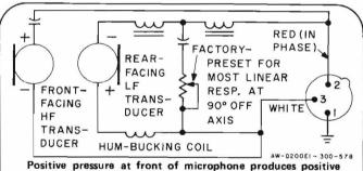
Positive pressure at front of microphone produces positive voltage on pin 2 from both transducers. (Though connected out of phase, they face in opposite directions, thus operating in phase.)
