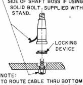
TO ROUTE CABLE THRU BOTTOM OF SHAFT BOSS & OUT THRU REAR OF STAND, USE HOLLOW-CENTER BOLT SUPPLIED WITH MICROPHONE & BREAK OUT TAB(S) AT REAR OF STAND.
