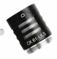
Ultra Linear Series cardioid capsule for use with C 460 B. Diaphragm diameter about 15 mm (0.6 in.) Same applications as for CK 1, especially suited for difficult sources thanks to excellent response
