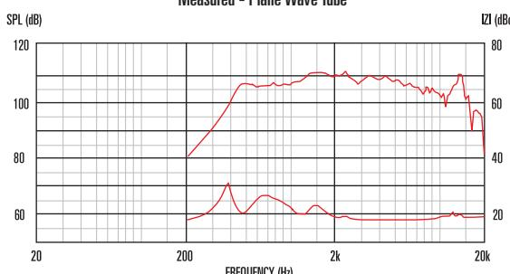
1. Tested for two hours on plane wave tube using a continuous, band-limited pink noise signal as per AES standard. Power calculated on minimum impedance.
