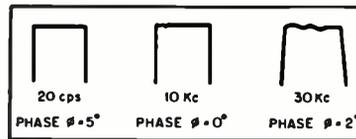
Fig. 7. Square-wave performance of the Ultra-Linear amplifier.
