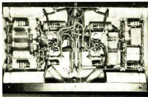
Fig. 9. Underside of dividing network chassis.
