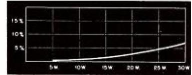
Fig. 3. Intermodulation distortion vs. power output.
