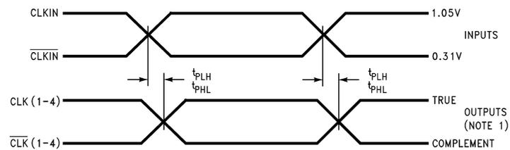
**Figure 4. Propagation Delay, CLKIN/CLKIN to Outputs**
