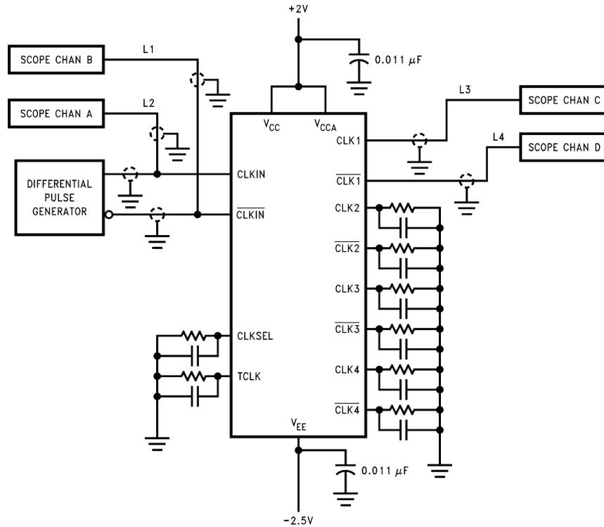
Shown for testing CLKIN to CLK1 in the differential mode.
