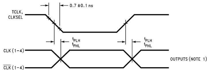
**Figure 3. Propagation Delay, TCLK, CLKSEL to Outputs**
