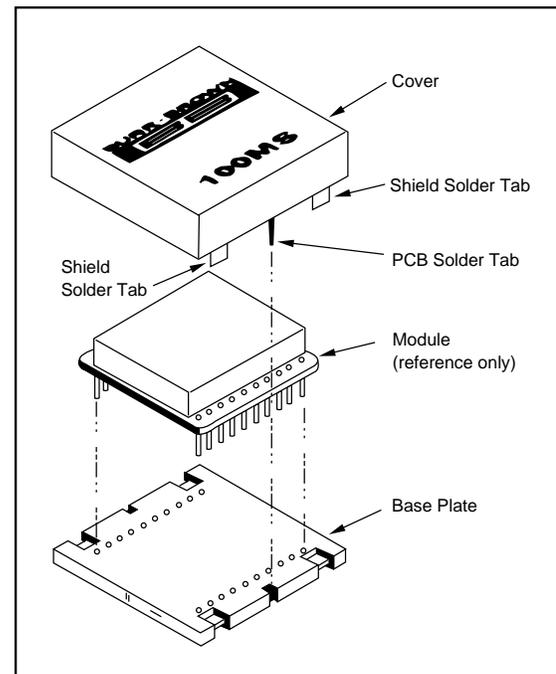
FIGURE 2. Assembly Diagram.
