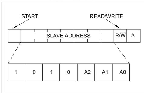
**FIGURE 3-3: ADDRESS SEQUENCE BIT ASSIGNMENTS**
