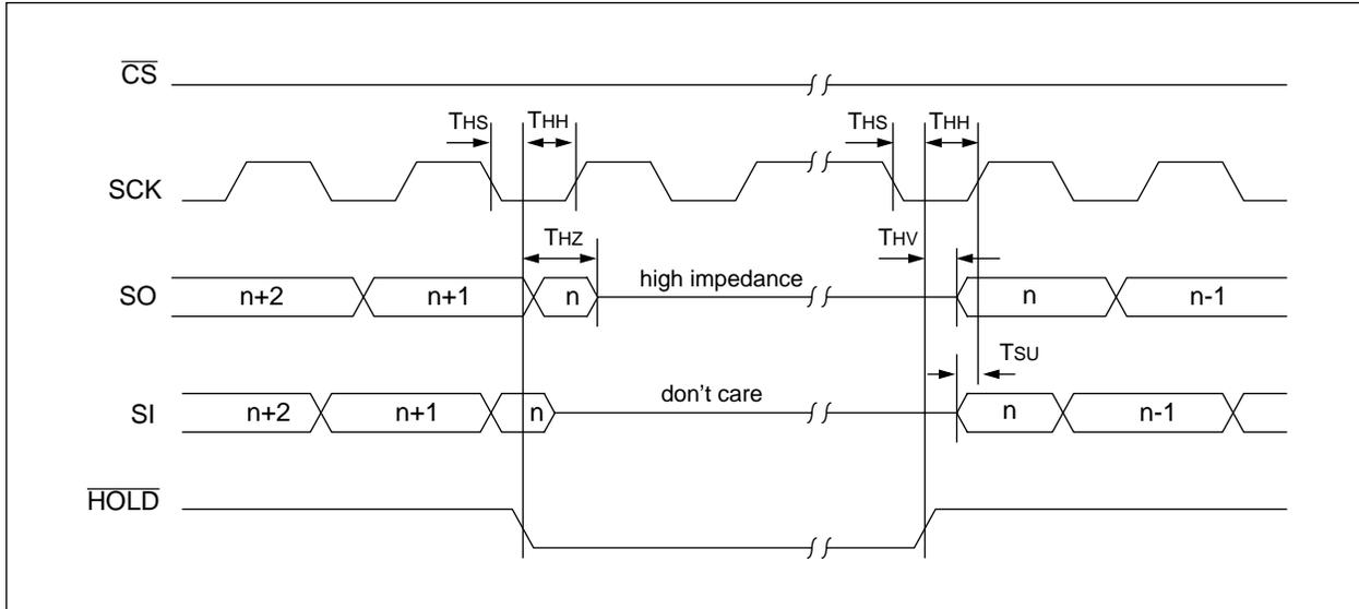
**FIGURE 1-3: SERIAL INPUT TIMING**
