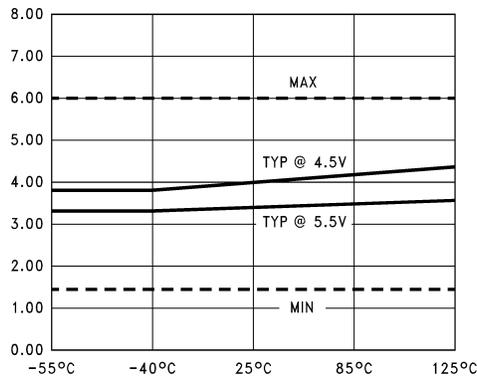
**Figure 10.  $t_{PLZ}$  vs Temperature ( $T_A$ )**
