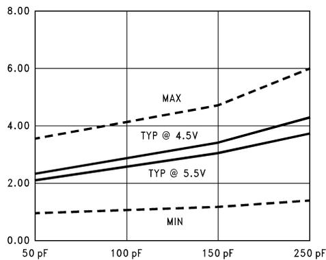
**Figure 6.  $t_{PHL}$  vs Load Capacitance
