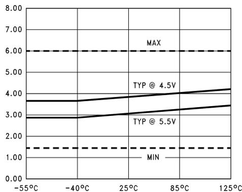
**Figure 12.  $t_{PHZ}$  vs Temperature ( $T_A$ )**
