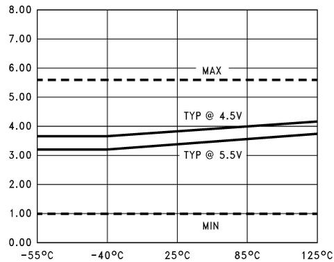
**Figure 13.  $t_{PHZ}$  vs Temperature ( $T_A$ )**
