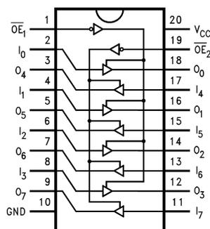
**Figure 2. Pin Assignment for LCC**
