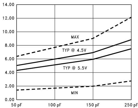
**Figure 18.  $t_{PZH}$  vs Load Capacitance
