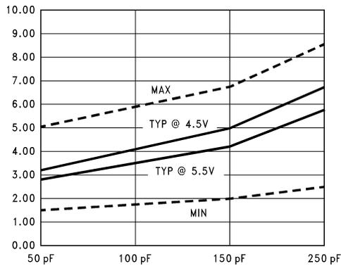
**Figure 8.  $t_{PHL}$  vs Load Capacitance
