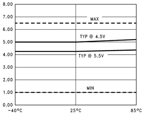
**Figure 16.  $t_{PZL}$  vs Temperature ( $T_A$ )
