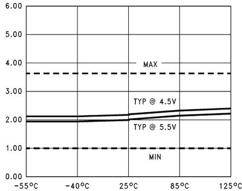
Figure 4.  $t_{PHL}$  vs Temperature ( $T_A$ )
