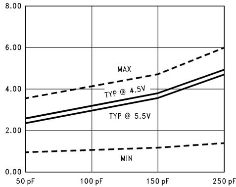
**Figure 7.  $t_{PLH}$  vs Load Capacitance
