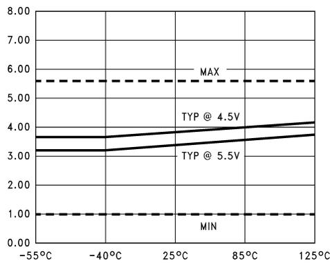
**Figure 11.  $t_{PZH}$  vs Temperature ( $T_A$ )**
