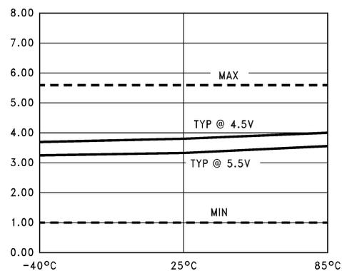
**Figure 15.  $t_{PZL}$  vs Temperature ( $T_A$ )
