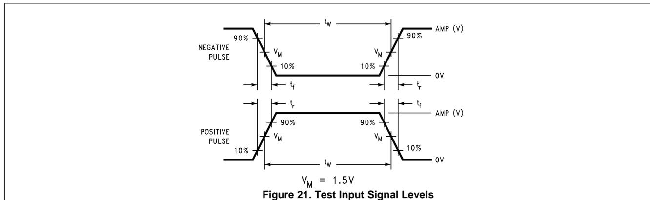
Test Input Signal Requirements
