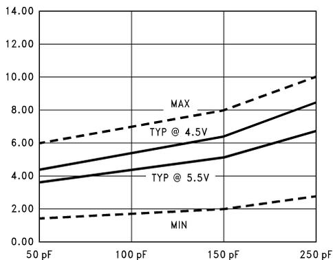
**Figure 19.  $t_{PLH}$  and  $t_{PHL}$  vs Number
