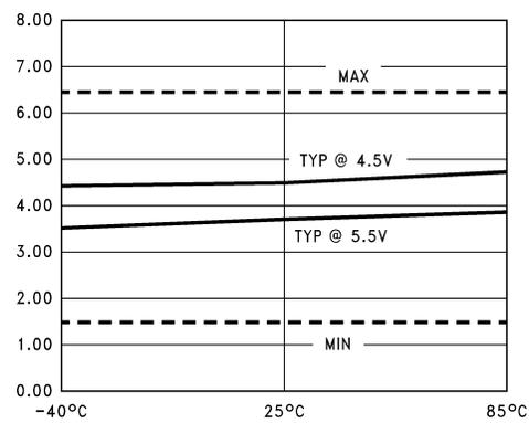
**Figure 14.  $t_{PHZ}$  vs Temperature ( $T_A$ )**
