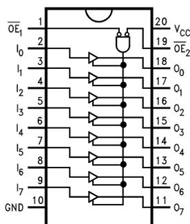
Figure 2. Pin Assignment
