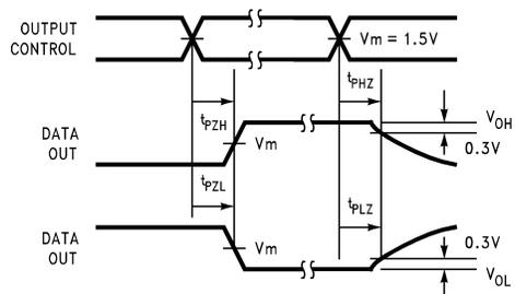
**Figure 24. TRI-STATE Output HIGH and LOW Enable and Disable Time**
