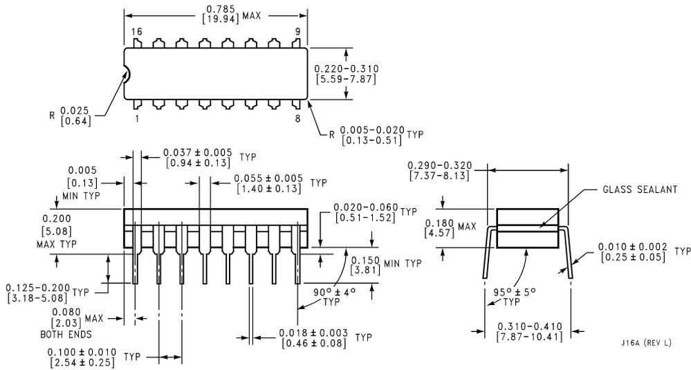
**16 Lead Ceramic Dual In-Line Package (D)**
