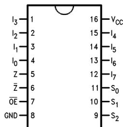
**Figure 3. Pin Assignment for LCC**
