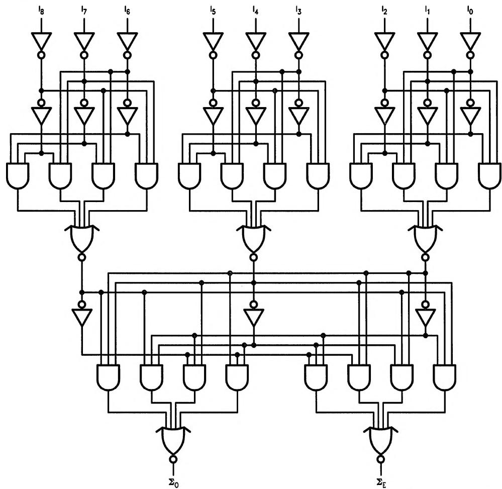
Please note that this diagram is provided only for the understanding of logic operations and should not be used to estimate propagation delays.
