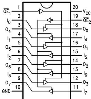
Figure 2. Pin Assignment for DIP and Flatpak
