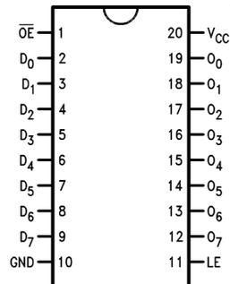
**Figure 3. Pin Assignment for LCC**
