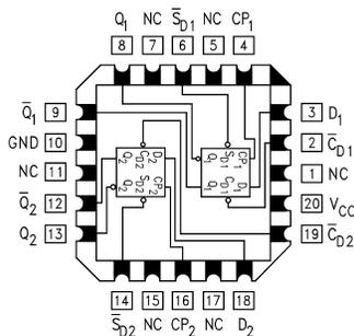
Figure 3. Pin Assignment for LCC
