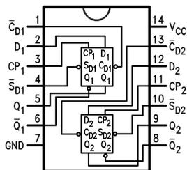
Figure 2. Pin Assignment for DIP and Flatpak
