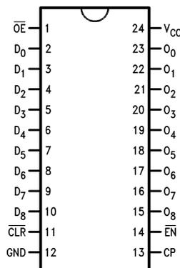
**Figure 3. Pin Assignment for LCC**
