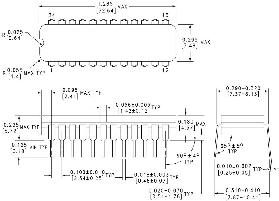
**24-Lead Slim (0.300" Wide) Ceramic Dual-In-Line Package (SD)**
