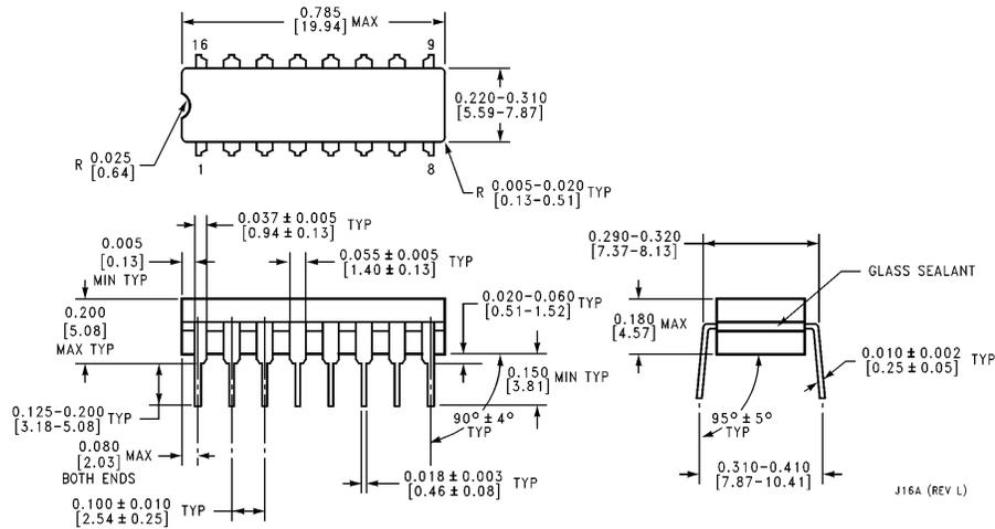
**16-Lead Ceramic Dual In-Line Package (D)**
