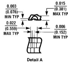
**20-Lead Ceramic Leadless Chip Carrier (L)**
