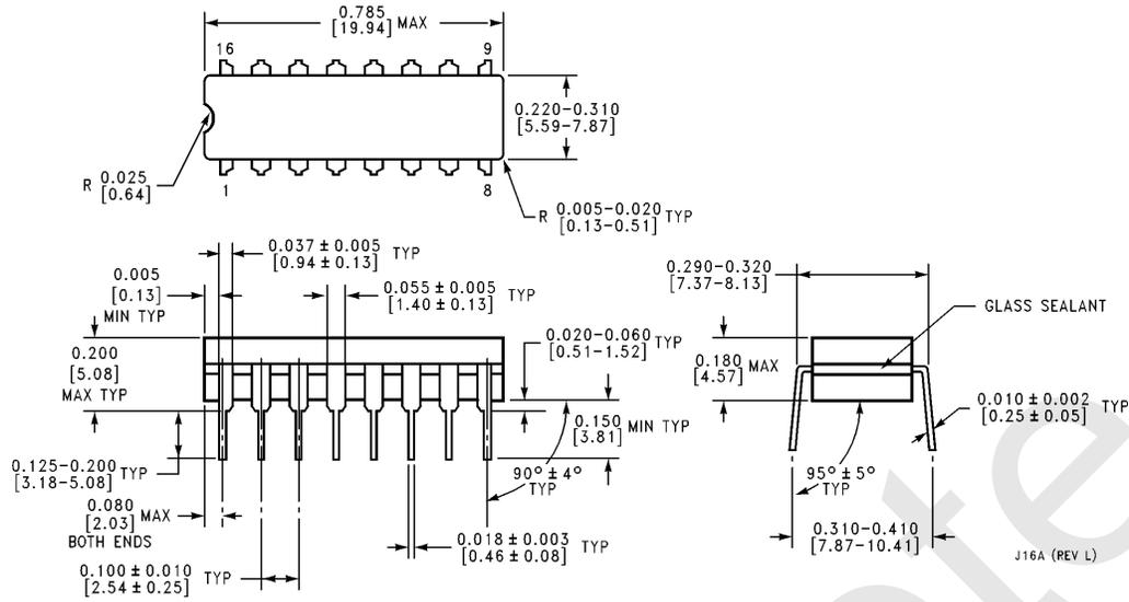
**16-Lead Ceramic Dual-In-Line Package (D)
