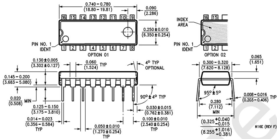
**16-Lead (0.300" Wide) Molded Dual-In-Line Package (P)**
