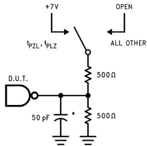
\*Includes jig and probe capacitance
