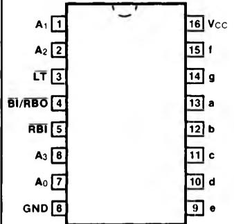
**DESCRIPTION** — The 'LS249 has active HIGH open-collector outputs and is the 16-pin version of the 14-pin 'LS49. The 'LS249 incorporates the Lamp Test and BI/RBO inputs that are omitted in the 'LS49. Additionally, the 'LS249 will light the top bar (segment a) for numeral 6 and the bottom bar (segment d) for numeral 9. For detailed description and specifications please refer to the 'LS49 data sheet.
