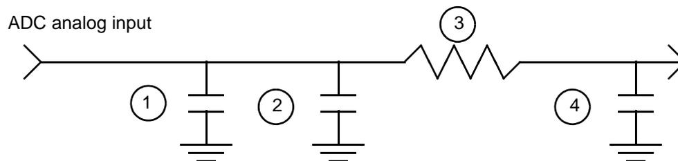
1. Parasitic capacitance due to package, pin to pin, and pin to package base coupling. (1.8pf)
