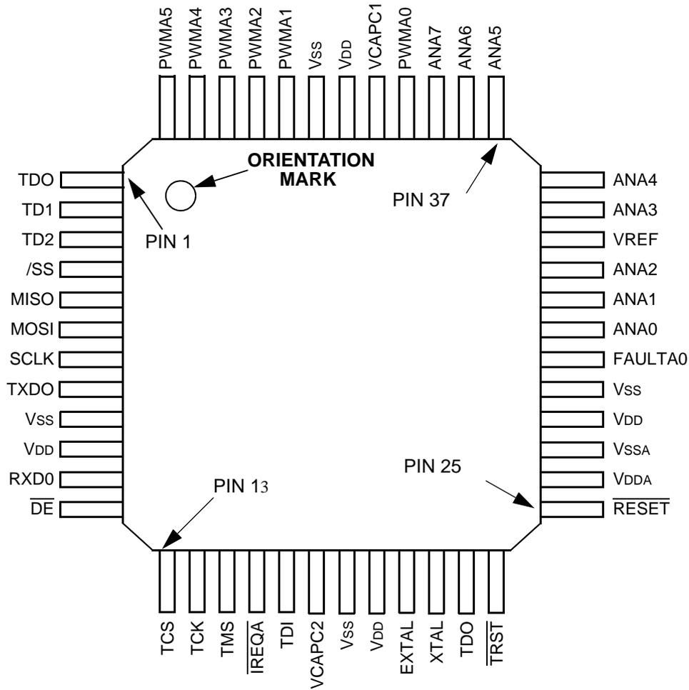
**Figure 4-1 Top View, 56F801 48-pin LQFP Package**
