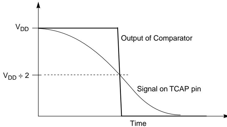
**Figure 9-8. TCAP Input Comparator Output**
