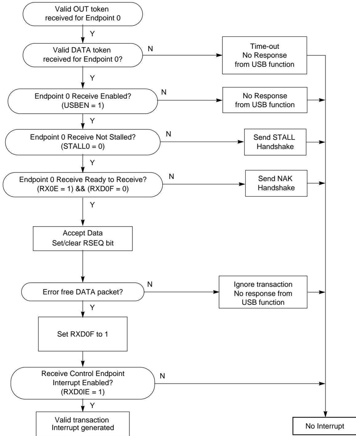
**Figure 10-29. OUT Token Data Flow for Receive Endpoint 0**
