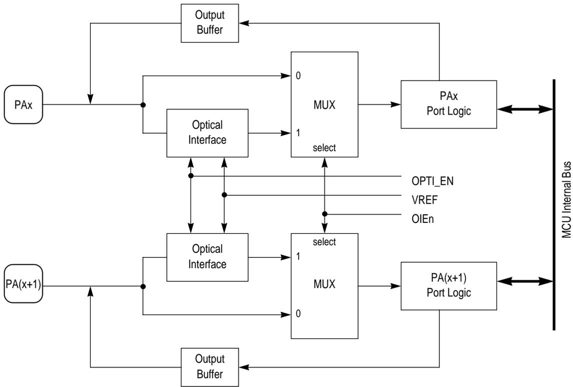
**Figure 11-1. A pair of Optical Coupler Interface**
