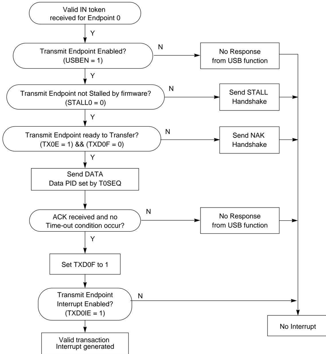
**Figure 10-31. IN Token Data Flow for Transmit Endpoint 0**
