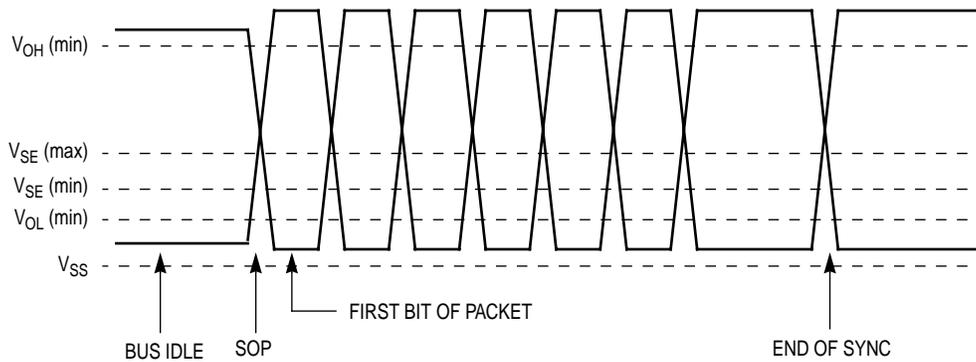
**Figure 10-5. SOP, Sync Signaling and Voltage Levels**
