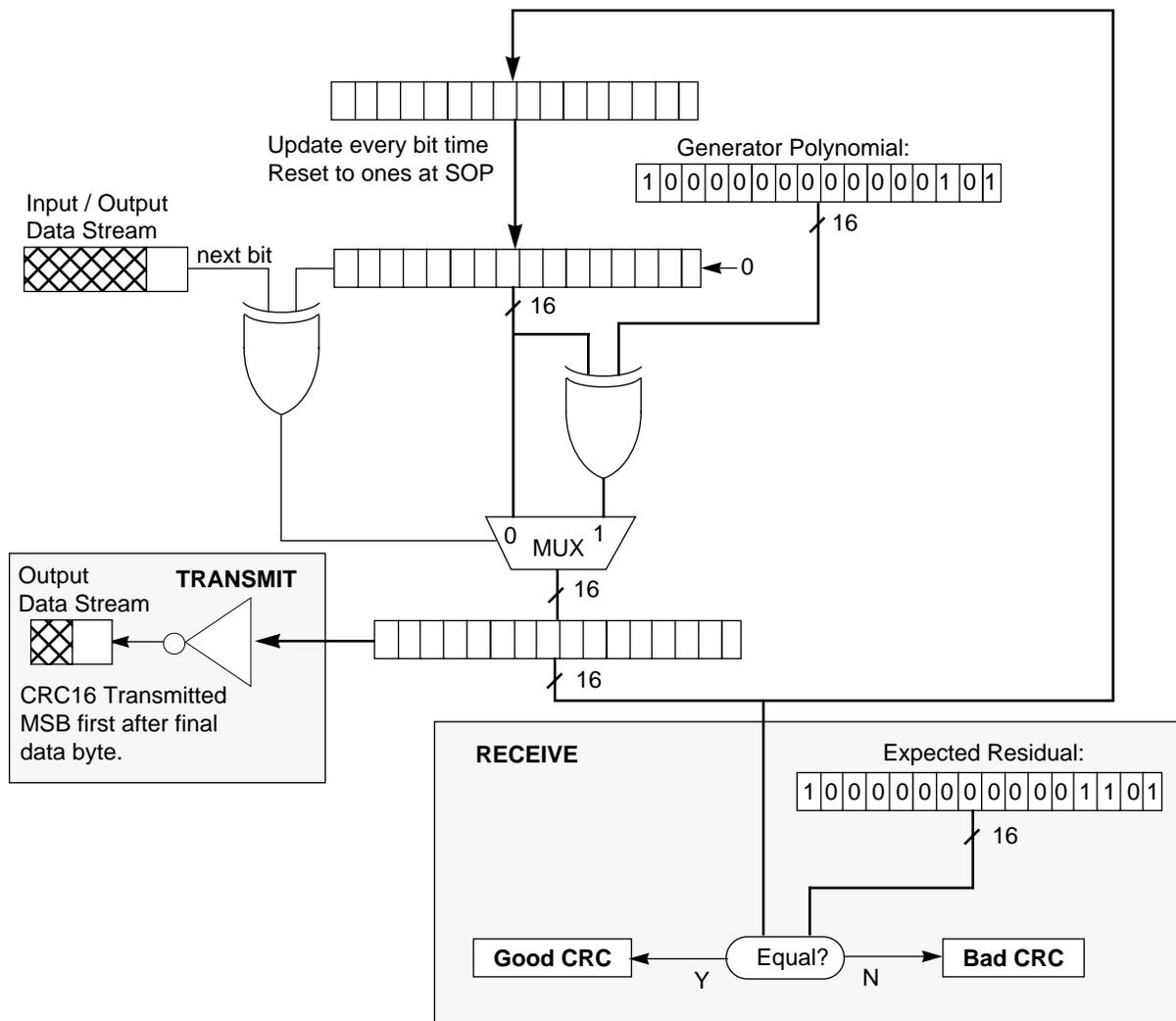
Figure 10-7. CRC Block Diagram for Data Packets
