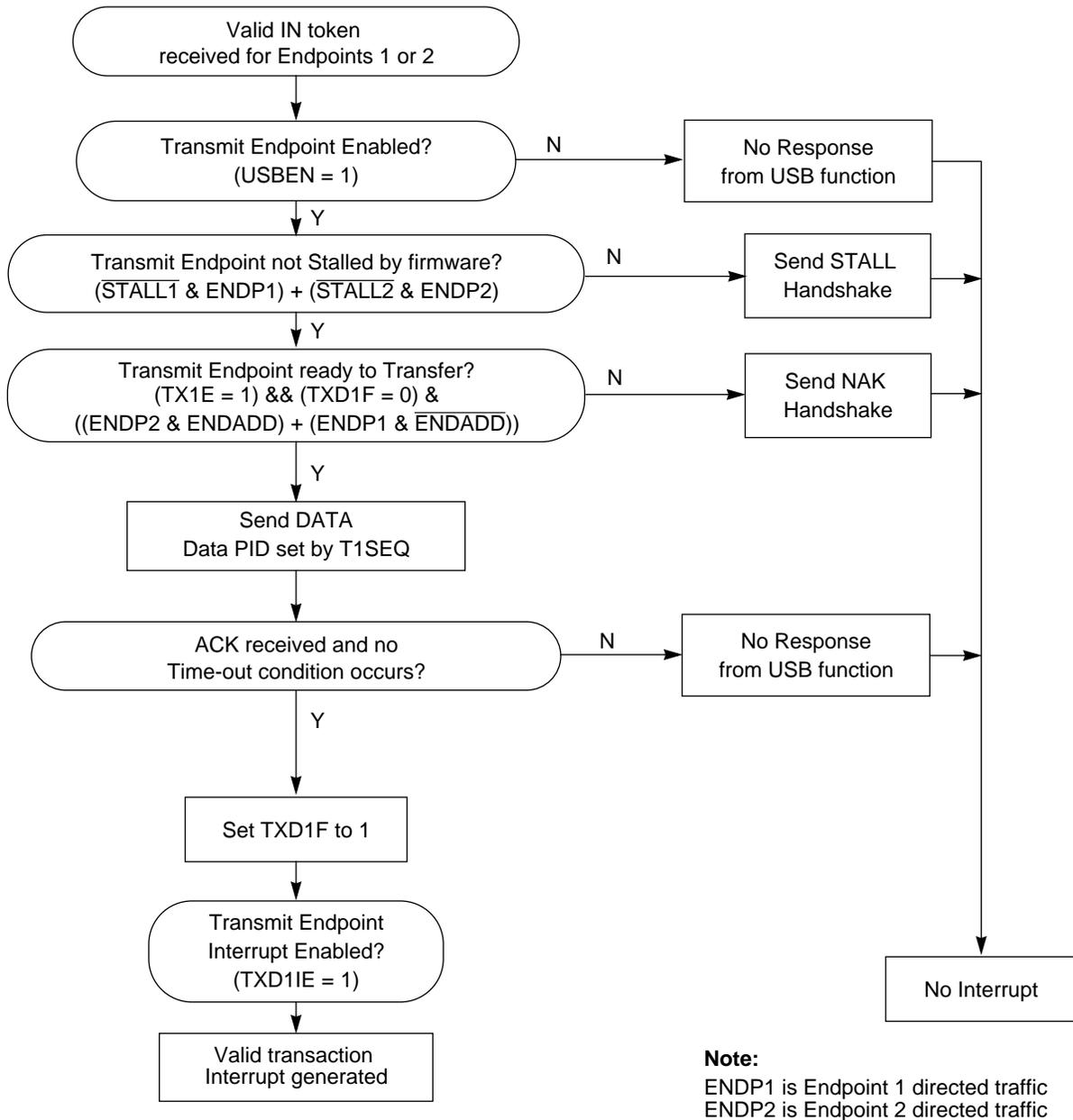
**Figure 10-32. IN Token Data Flow for Transmit Endpoint 1/2**
