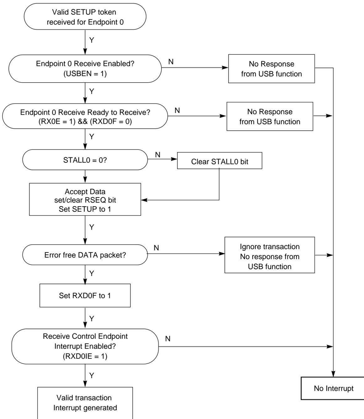
**Figure 10-30. SETUP Token Data Flow for Receive Endpoint 0**
