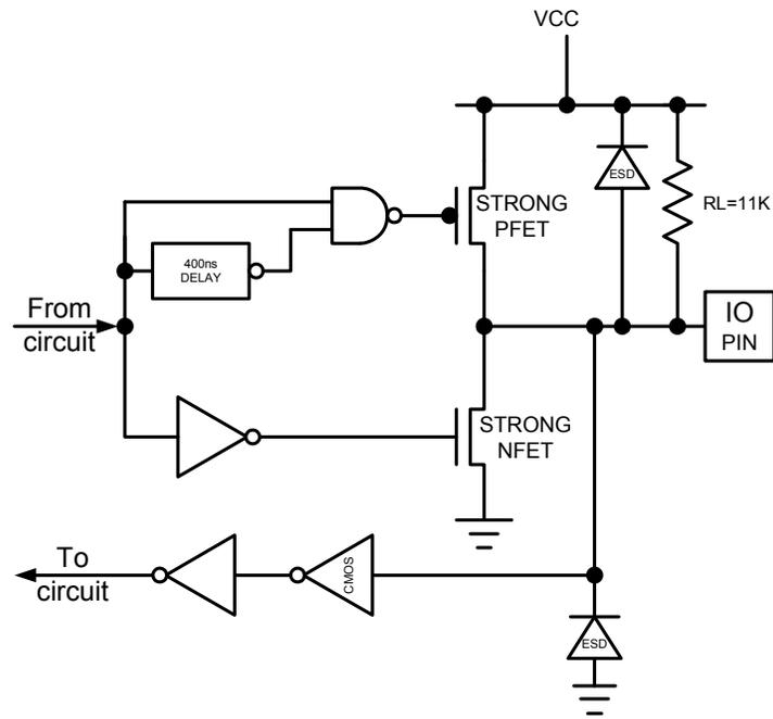
Figure 14: Type 7A – Smart Card IO Interface Circuit
