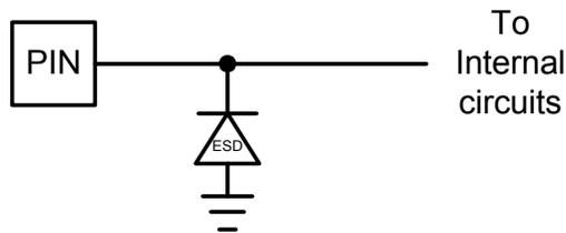
Figure 11: Power Input/Output Circuit,  $V_{DD}$ ,  $V_{PC}$ ,  $V_{CC}$
