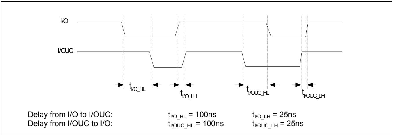
Figure 9: I/O - I/OUC Delays - Timing Diagram
