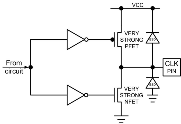
Figure 12: Type 5 – Smart Card CLK Driver Circuit
