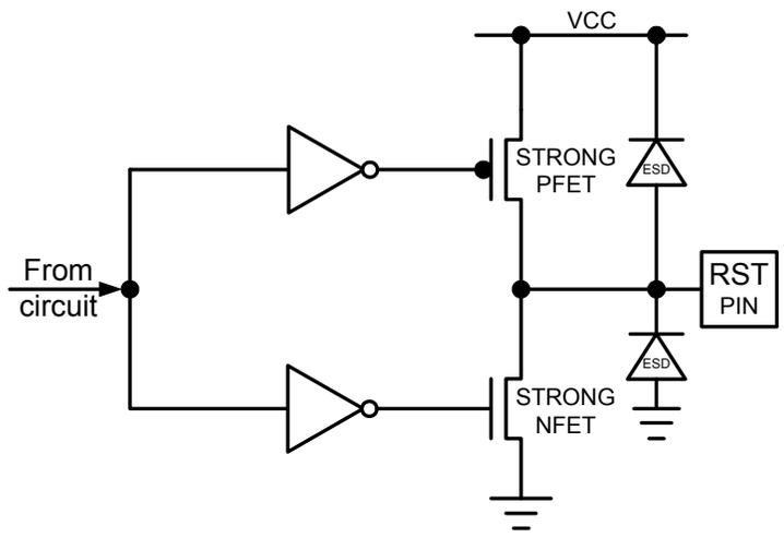
Figure 13: Type 6 – Smart Card RST Driver Circuit
