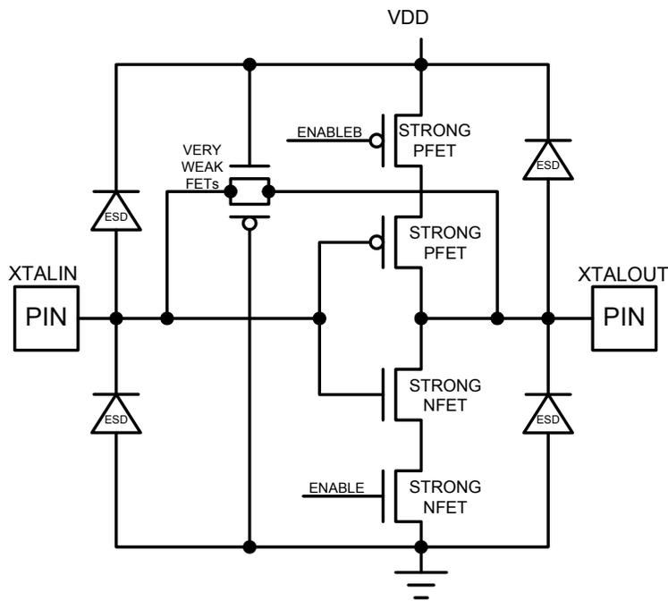
Figure 17: Oscillator Circuit
