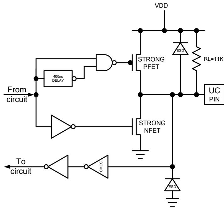
Figure 15: Type 7B – Smart Card IOUC Interface Circuit
