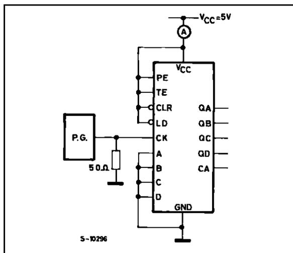
TOTAL OPERATING CURRENT WHEN USING A CAPACITIVE LOAD
