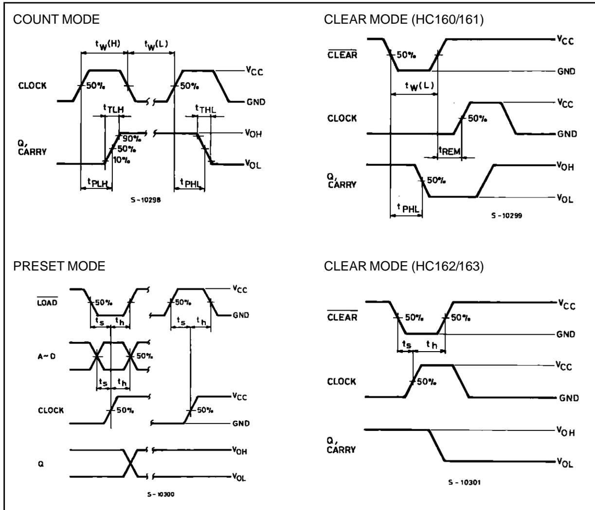
SWITCHING CHARACTERISTICS TEST WAVEFORM (continued)
