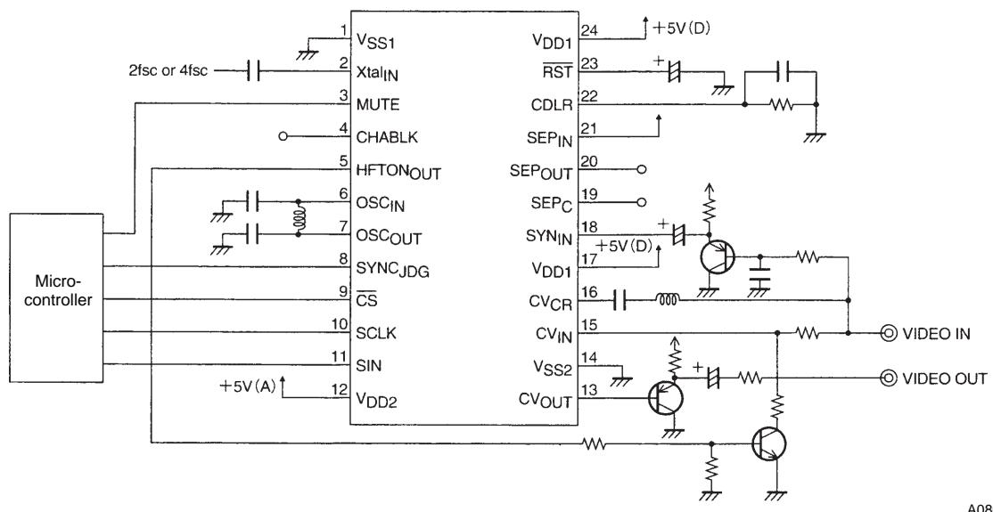
Note: When a sync tip level of 1.3 V DC (CV<sub>IN</sub> input signal: sync tip = 1.3 V) is selected for the internal generated video signals by option settings, the electrolytic capacitor connected to SYNIN must be connected with the correct polarity.
