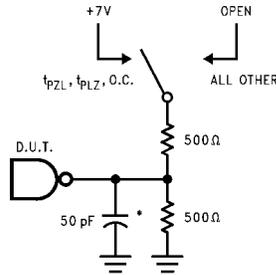
\*Includes jig and probe capacitance
