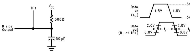
FIGURE 4. A to B Direction Test Load and Waveforms for Open Drain B<sub>1</sub> - B<sub>7</sub>
