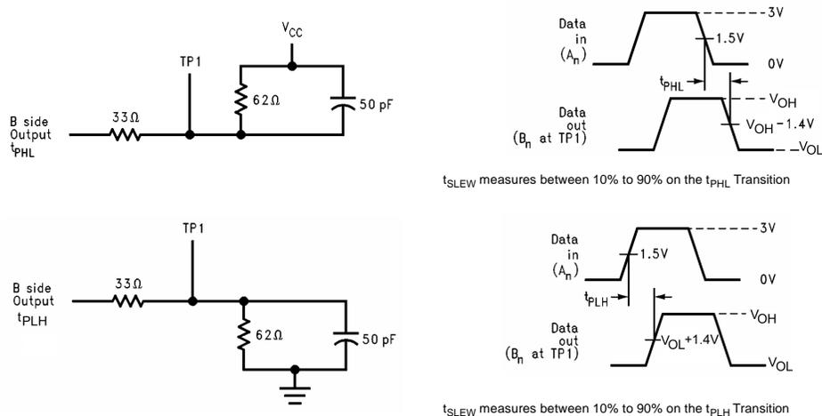
FIGURE 1. Port A to B Propagation Delay Waveforms
