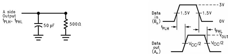
FIGURE 3. B to A Direction Test Load and Waveforms for Outputs A<sub>1</sub> - A<sub>4</sub>
