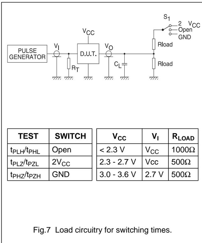
NOTES:  $V_{CC} = 2.3$  TO  $2.7$  V RANGE AND  $V_{CC} < 2.3$  V
