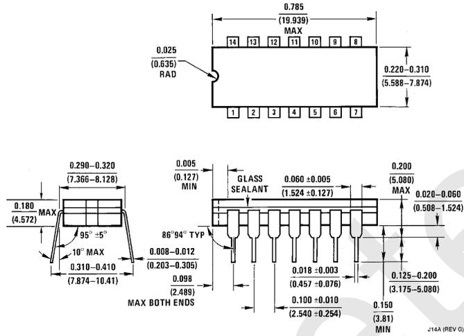
**14-Lead Ceramic Dual-In-Line Package (D)**
