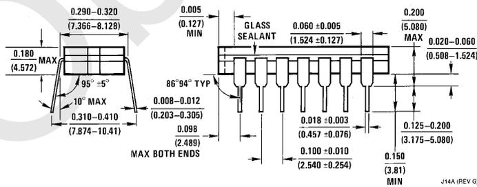
**14-Lead Ceramic Dual-In-Line Package (D)**
