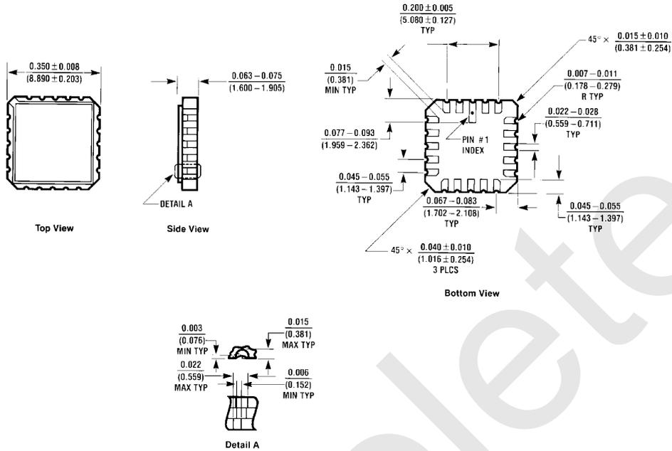
**20-Lead Ceramic Leadless Chip Carrier (L)**
