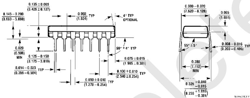
**14-Lead (0.300" Wide) (Molded Dual-In-Line Package (P))**
