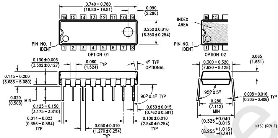
**16-Lead (0.300" Wide) Molded Dual-In-Line Package (P)**
