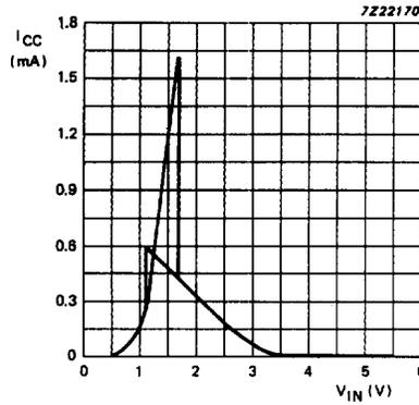
Fig.12 Typical HCT transfer characteristics;  $V_{CC} = 5.5 V$ .
