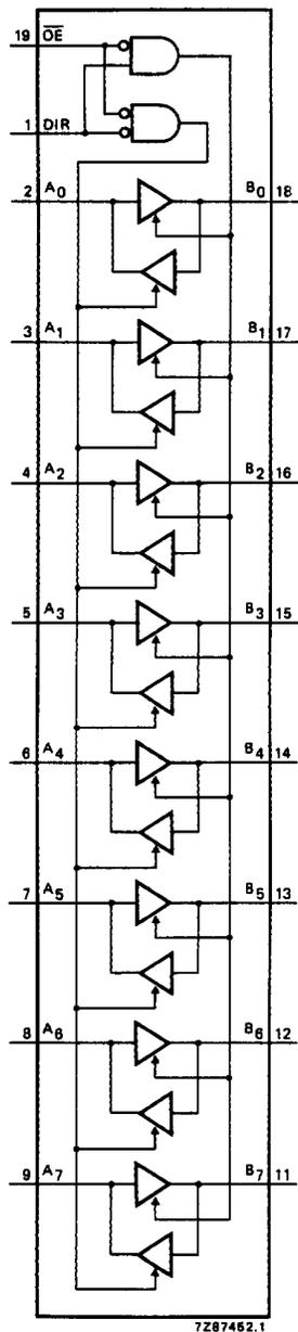
Fig.4 Functional diagram.
