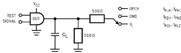
**FIGURE 1. AC Test Circuit (C<sub>L</sub> includes probe and jig capacitance)**
