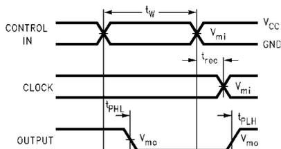
**Propagation Delay, Pulse Width and t<sub>rec</sub> Waveforms**
