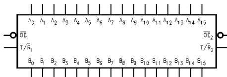
74VCX164245 Low Voltage 16-Bit Dual Supply Translating Transceiver with 3-STATE Outputs
