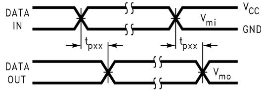
FIGURE 4. Waveform for Inverting and Non-Inverting Functions
