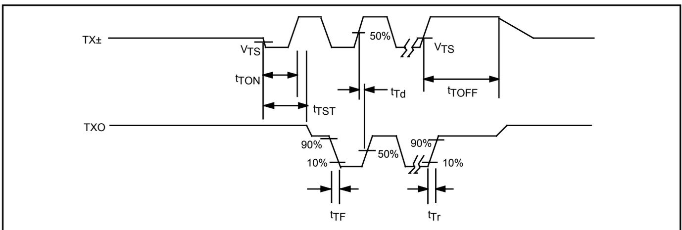
FIGURE 4: Transmitter Timing
