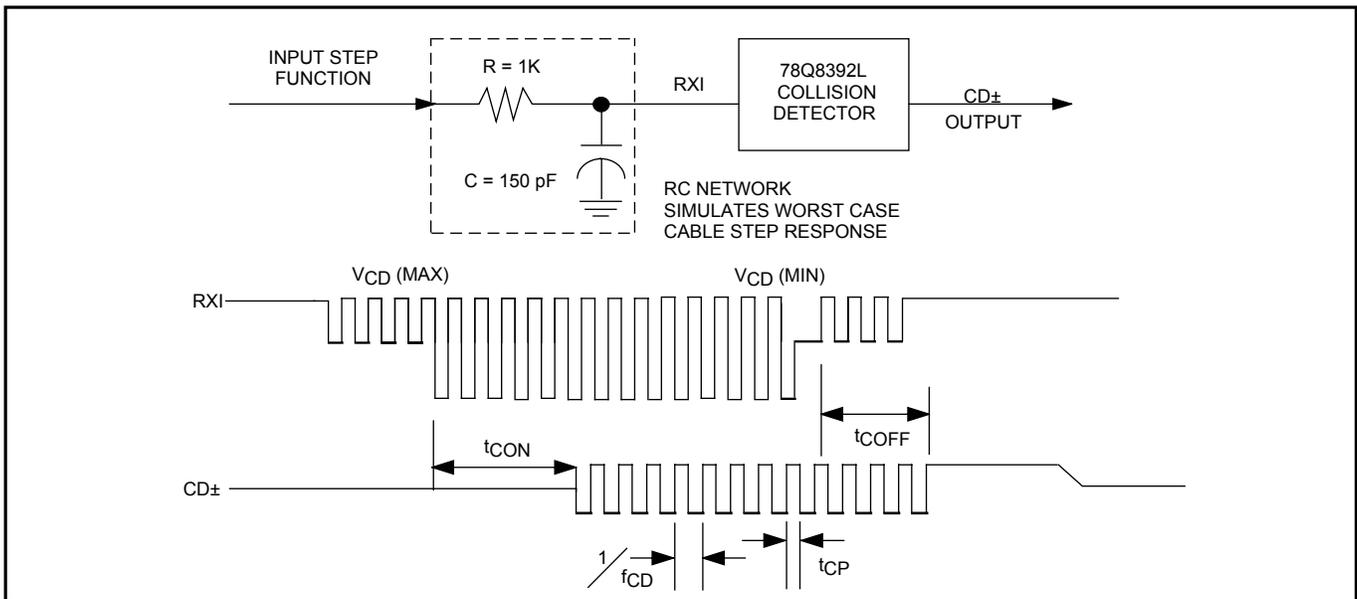
**FIGURE 5: Collision Timing**
