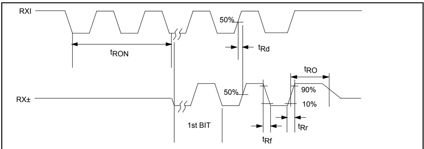
FIGURE 3: Receiver Timing
