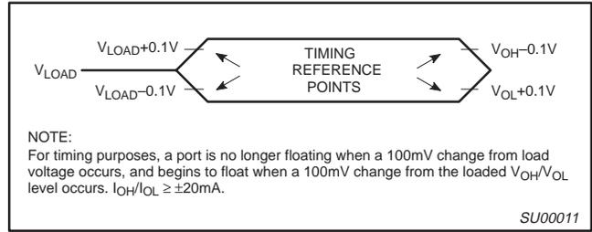
Figure 11. Float Waveform
