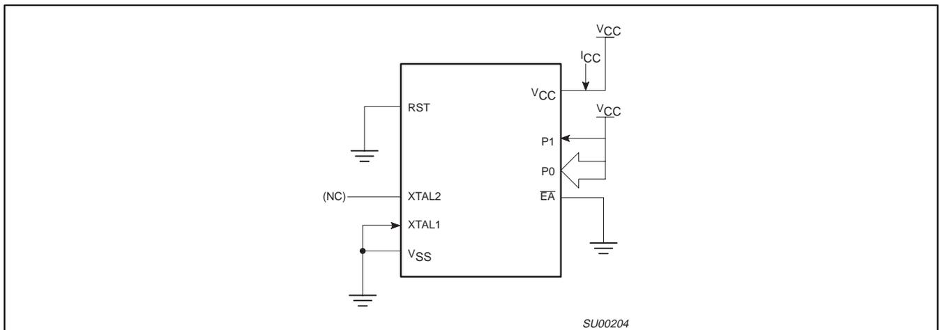
**Figure 16.  $I_{CC}$  Test Condition, Power Down Mode**
