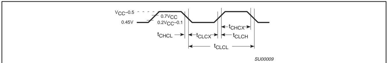
**Figure 15. Clock Signal Waveform for  $I_{CC}$  Tests in Active and Idle Modes**
