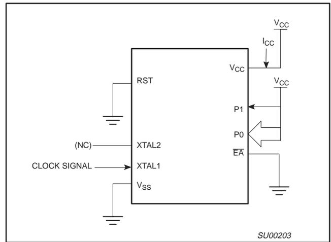
**Figure 14.  $I_{CC}$  Test Condition, Idle Mode**
