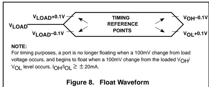
Figure 8. Float Waveform
