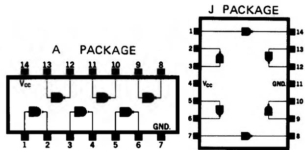
The 8H90 Hex Inverter is designed for ultra-high switching speed while maintaining high fan-out and noise margin.
