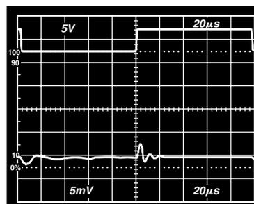
Figure 15. Load Transient Response (0 mA to -1 mA Load)
