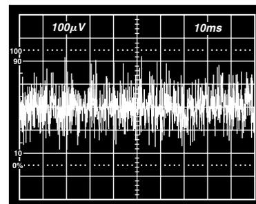
Figure 11. 10 Hz to 10 kHz Wideband Noise
