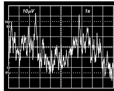
Figure 10. 0.1 Hz to 10 Hz Voltage Noise
