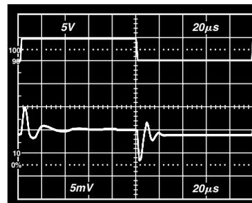
Figure 14. Load Transient Response (0 mA to 5 mA Load)
