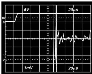
Figure 12c. Turn-On Settling
